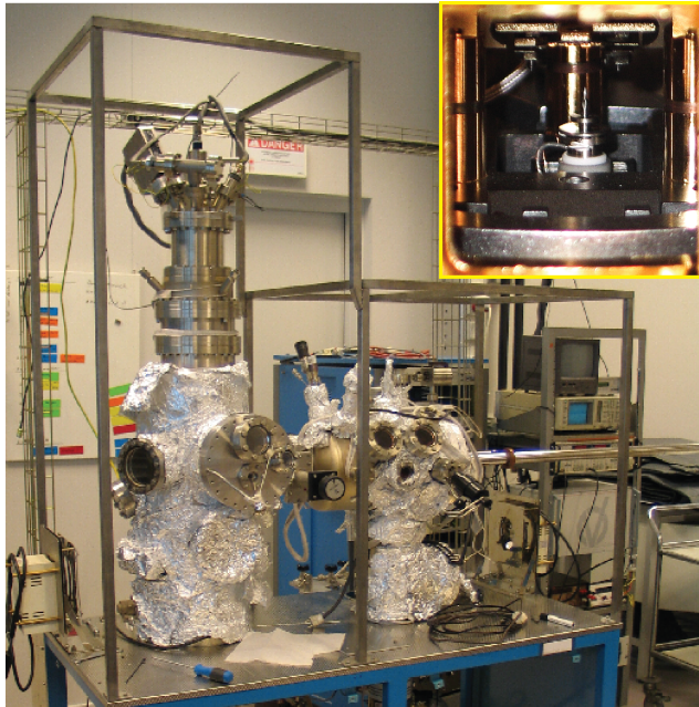
Figure 2.3: Photo of the LT-STM UHV system, located in the same MESA+ nanolab. The inset shows the STM-tip (bottom) and the sample (top).
